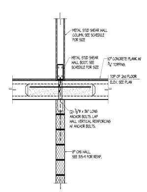
Figure 3. Second floor metal stud wall bearing on First floor CMU bearing walls
