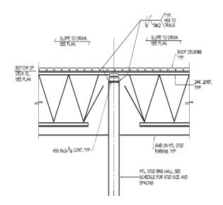
Figure 4 – Steel Joist Bearing on Metal Stud Wall
