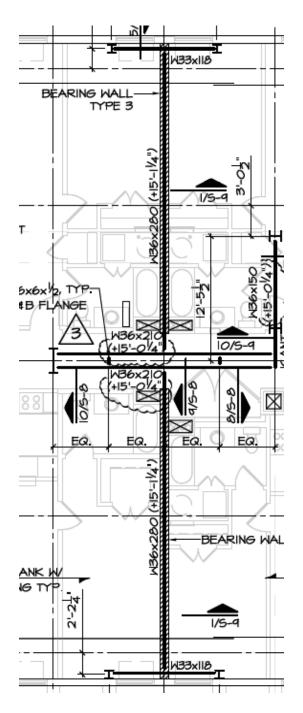
Figure 2 – Second Floor Transfer Beam Framing
