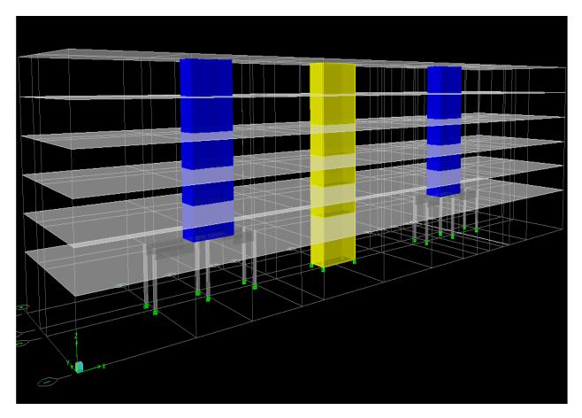
Figure 10 - Isometric of Lateral Resisting System Present in Pearl Condominiums
